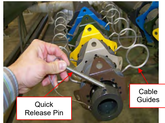
Figure 4-17 Install the Manual Position or Top Tube Stub
