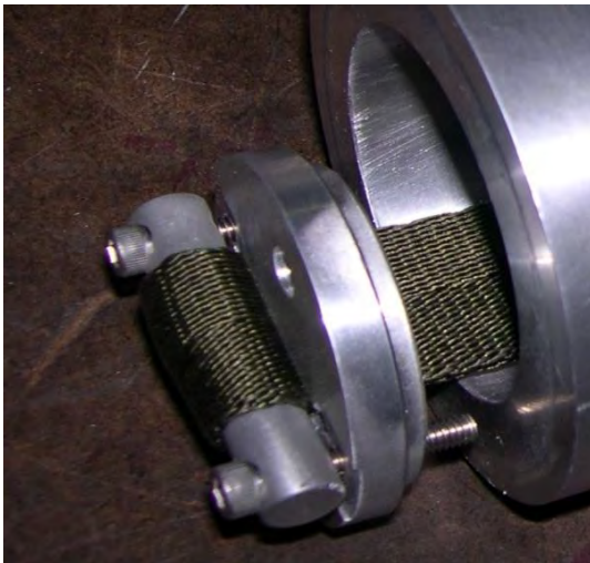
Figure 7-8 Pull Out the Top Stub Cap
