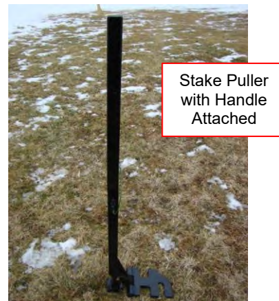
Figure 5-13 Press Blue Button Then Insert the Pin to Connect Handle
