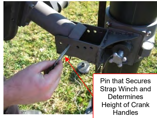
Figure 4-23 Secure Winch at Desired Position
