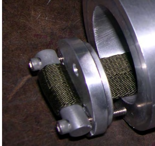
Figure 7-10 Secure Strap Pin in Place
