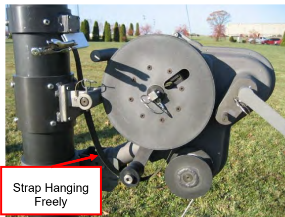
Figure 8-4 Crank Winch in Reverse Direction to Transfer Load from Winch to Clamp Block
