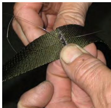
Figure 7-3 Create a Butt Splice
