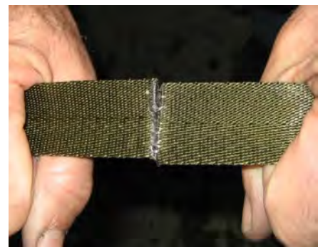
Figure 7-4 Test the Splice
