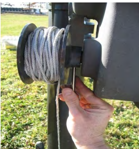
Figure 4-24 Attach Positive Retraction Reel to Strap Winch
