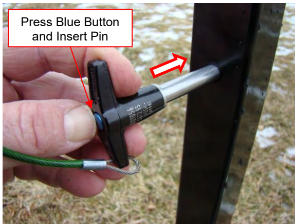
Figure 5-13 Press Blue Button Then Insert the Pin to Connect Handle
