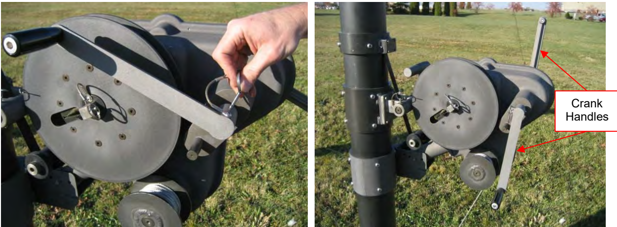
Figure 4-27 Attach Crank Handles to the Strap Winch at the Desired Reduction Shafts and 180° apart
