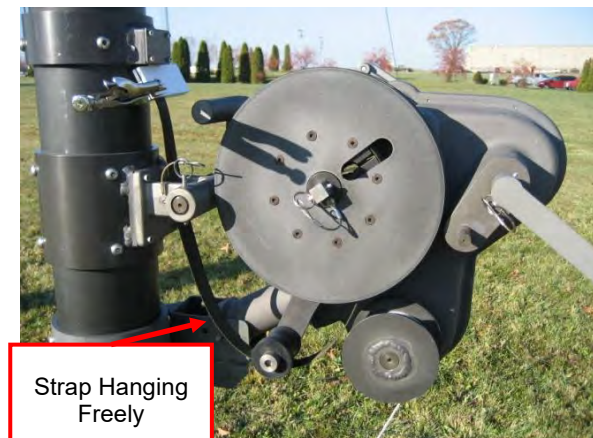
Figure 8-2 Crank Winch in Reverse Direction
