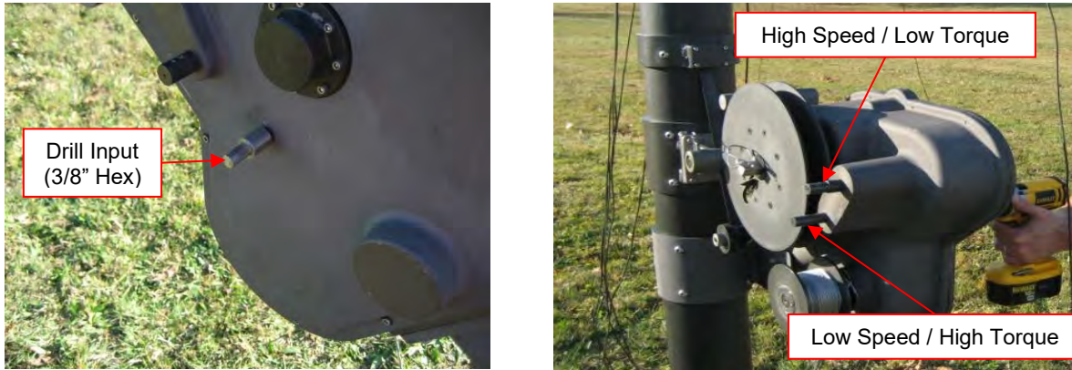
Figure 4-28 When Using Cordless Drill to Extend Mast, Set Drill to Lowest Torque that Will Operate Mast
