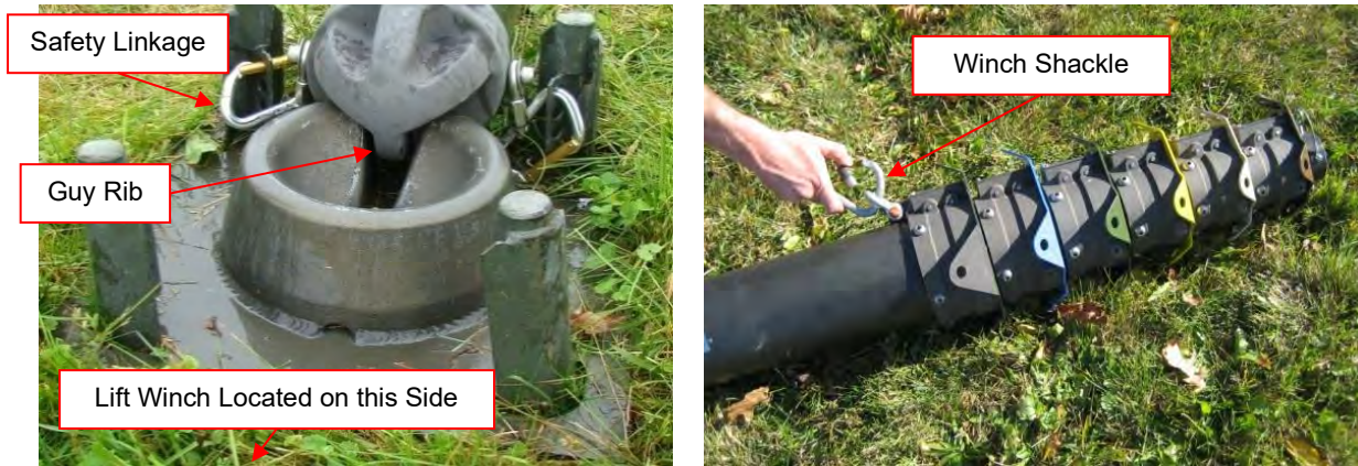
Figure 4-6 Place the Base of the Mast on the Base Plate
