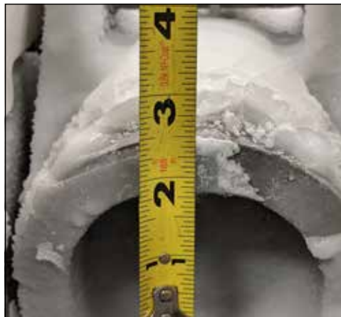
The Night Scan Powerlite IQ was tested at -15° F (-26° C) with a ¼" (6mm) of ice
