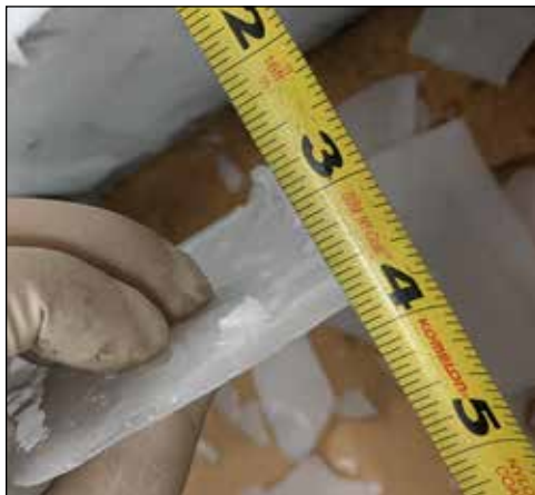
The Night Scan Powerlite IQ was tested at -15° F (-26° C) with a ¼" (6mm) of ice
