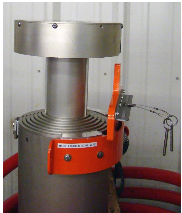
Clamp and Vertical Support on Mast
