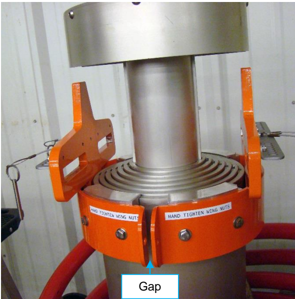
Both Clamps and Vertical Support On Mast
