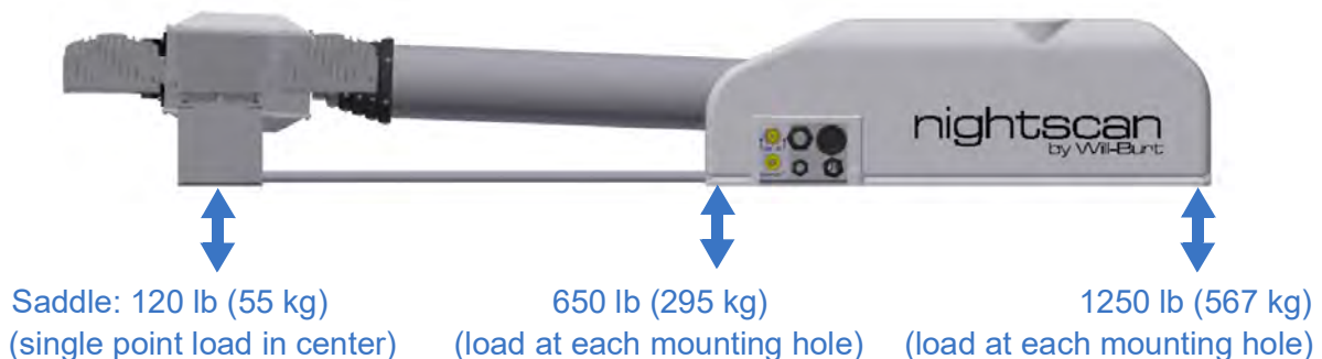
Figure 5-1 Reaction Loads on Mounting Structure
