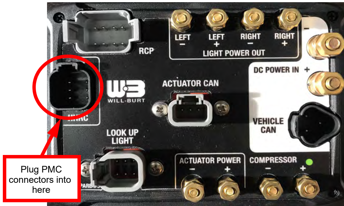
Figure 5-6 Plug PMC Connectors Into Matching I/O Module Connectors
