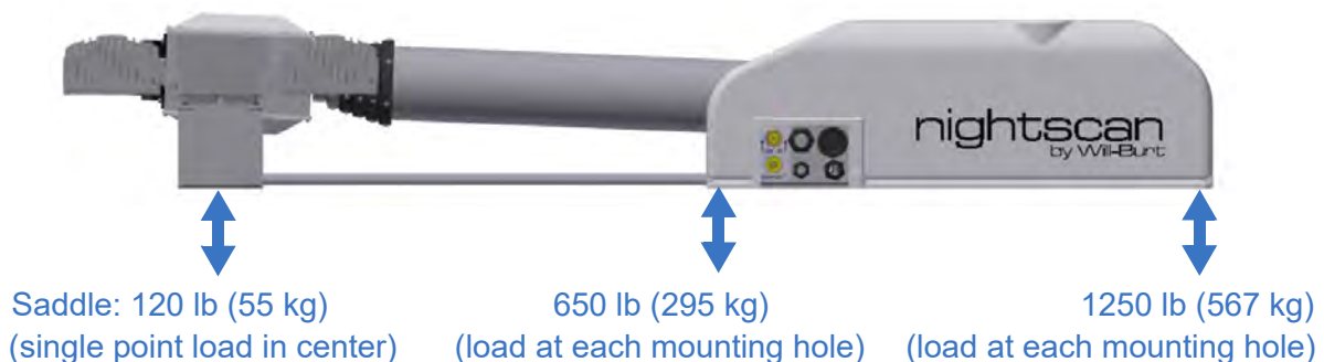
Figure 5-1 Reaction Loads on Mounting Structure
