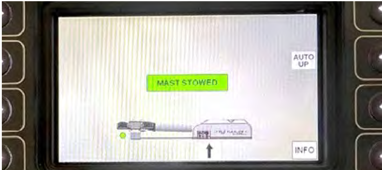
Figure 6-5 Mast is Fully and Properly Initiated Screen
